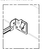
B. LOCK HANGER BARS USING PROVIDED SCREW
