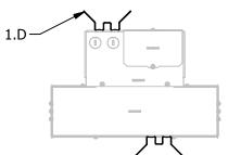
E. HANGER BAR BRACKET WILL WORK WITH STANDARD C-CHANNEL. FOR OTHER HANGER BAR OPTIONS, CONTACT AMERLUX
