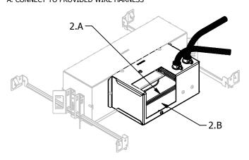
B. KEEP WIRES CONTAINED IN JUNCTION BOX AS CLOSE TO THE ACCESS PLATE AS POSSIBLE. LEAVE 6"-8" OF WIRE AND ENSURE THAT SPLICES ARE ACCESIBLE THROUGH CEILING CUTOUT.
