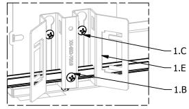
D. ALTERNATIVE MOUNTING FOR HANGER BAR BRACKETS SHOWN BELOW (LOOSEN SCREW AND REMOVE BRACKETS USING KEY SLOTS)
