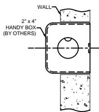
Install 2" x 4" J-box at feed location(s) 2" to 2 1/4" above where bottom edge of fixture is to be located above finished floor as shown above. For feed locations refer to *Longitudinal mounting points/feed detail* above and submittal layout(s).
