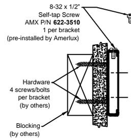
Orient wall mount support bracket with .128 hole & pre-installed screw UP as shown at left & below.
