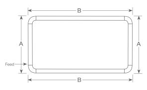
PR - Closed Rectangle, (4) straight lengths + (4) 90 corners Provide overall lengths: A' & B'; Diameter
