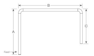
PU - Open U, (3) straight lengths + (2) corners Provide overall lengths: A', B' & C'; Diameter & Angle of corners Example: 4'x10'.D72xA45.PU
