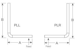
PLL - L Left, (2) straights + (1) corner, leg right PLR - L Right, (2) straights + (1) corner, leg left Provide overall lengths: A' & B'; Diameter & Angle of corner Example: 4'x8'.D43xA90.PLL
