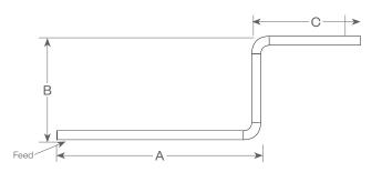
PZ - Open Z, (3) straight lengths + (2) corners Provide overall lengths: A', B' & C'; Diameter & Angle of corners Example: 12'x6'x10'.D36XA90.PZ
