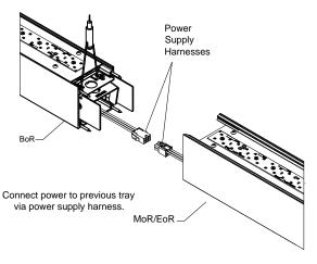
5. Align & join: Alignment pins Align (4) pins & press fit fixtures together Alignment pins MoR/EoR
