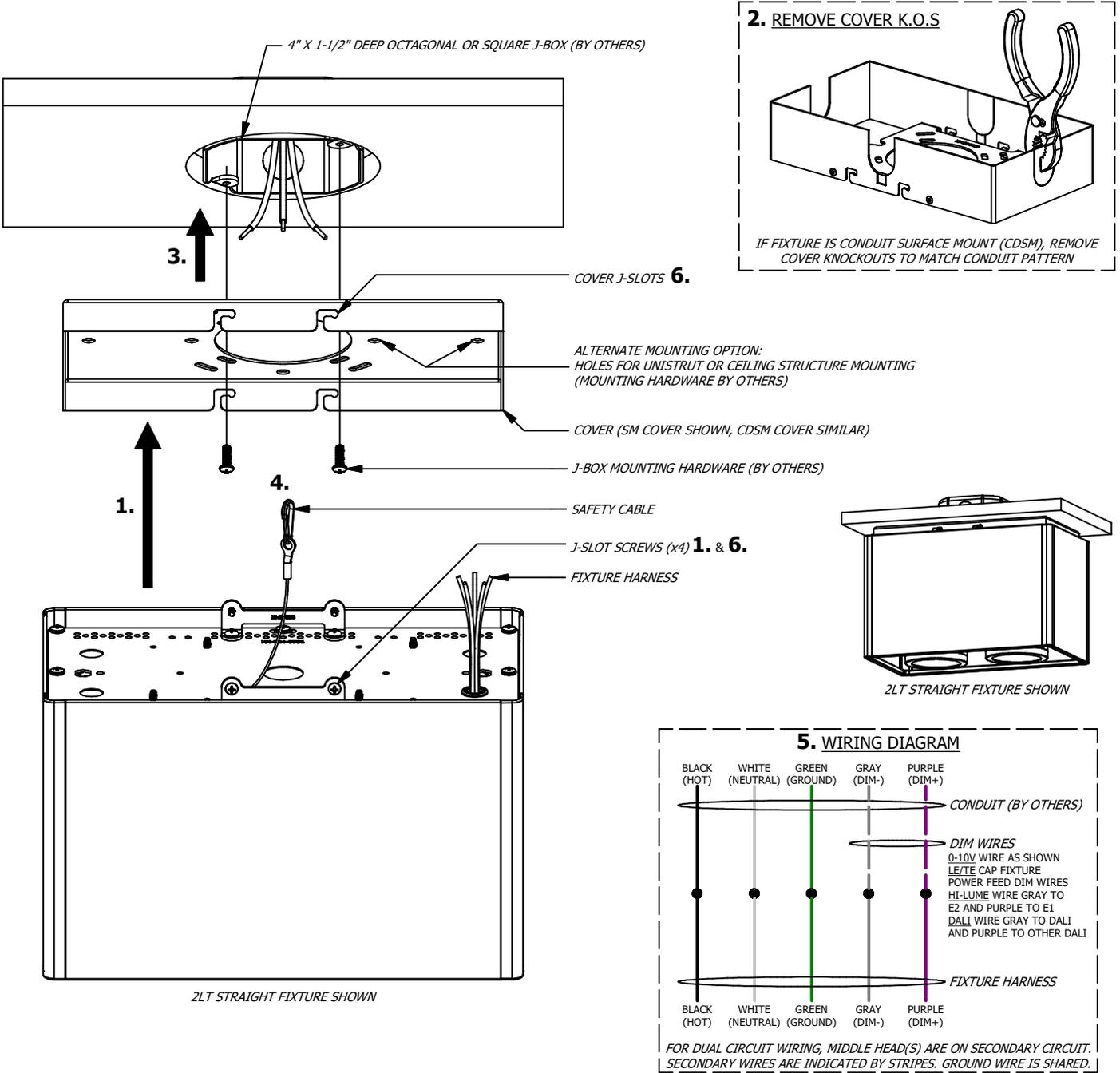
1. LOOSEN J-SLOT SCREWS & REMOVE COVER, 2. REMOVE COVER K.O.S (IF NECESSARY), 3. MOUNT COVER, 4. ATTACH FIXTURE SAFETY CABLE TO COVER SLOT, 5. WIRE ACCORDING TO LOCAL AND NATIONAL CODE, 6. LOCATE J-SLOT SCREWS IN COVER J-SLOTS, THEN FULLY TIGHTEN SCREWS.
