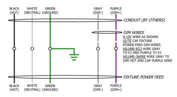
WIRE ACCORDING TO LOCAL AND NATIONAL CODE. CUT AND STRIP AS NEEDED. CAP UNUSED WIRES.
