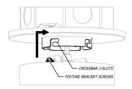
LOCATE FIXTURE BRACKET SCREWS IN CROSSBAR J-SLOTS, ROTATE UNTIL SCREWS ARE SEATED, THEN TIGHTEN SCREWS
