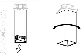
IF FIXTURE HAS WALL WASH TRIM AND/OR SQUARE HOUSING, SIMPLY ROTATE HOUSING (100° MAX.)
