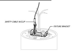
HOOK SAFETY CABLE CLIP ONTO FIXTURE BRACKET
