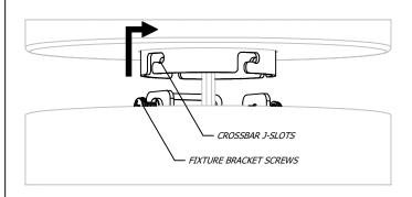
LOCATE FIXTURE BRACKET SCREWS IN CROSSBAR J-SLOTS, ROTATE UNTIL SCREWS ARE SEATED, THEN TIGHTEN SCREWS
