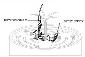
HOOK SAFETY CABLE CLIP ONTO FIXTURE BRACKET
