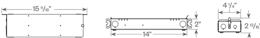
Driver is supplied installed in remote driver box, (one driver per box), with 15' of low voltage plenum rated cable. Amerlux recommends a maximum of 15' between the fixture and the remote driver box. Consult factory with job specific electrical spec if more than 15' is required.
