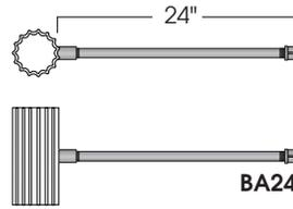
Fixed position banner arm for 4" or 5" OD poles (can be used on tapered poles). Aluminum 3/4" NPT coupling is permanently welded at the specified location. 24" extruded aluminum banner arm is removable.
