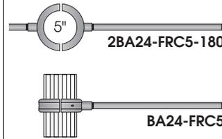
Single or double field rotatable arms for 5" OD non-tapered poles. 3/4" NPT x 24" long extruded aluminum arm threads onto cast collar that clamps to pole with (2) 3/8" dia. stainless steel socket head screws. Other lengths available.
