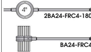
Single or double field rotatable arms for 4" OD non-tapered poles. 3/4" NPT x 24" long extruded aluminum arm threads onto cast collar that clamps to pole with (2) 3/8" dia. stainless steel socket head screws. Other lengths available.
