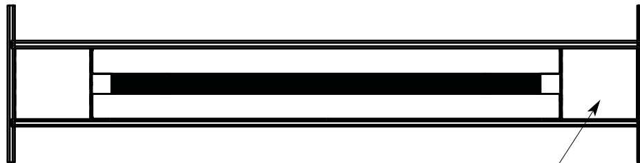
GRUV-IIV with 6" panels uses 3' lamps for 6"x4' and 4' lamps for 6"x5'
