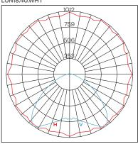
Maximum Candela = 1012 Located at Horizontal Angle = 60 Vertical Angle = 35 H - Horizontal Axial Candela V - Vertical Axial Candela **B1-U3-G1**
