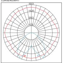
Maximum Candela = 1901 Located at Horizontal Angle = 340 Vertical Angle = 26 H - Horizontal Axial Candela V - Vertical Axial Candela B2-U3-G1
