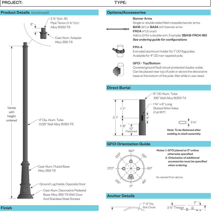
The post will be finished with an electrostatically applied thermoset polyester powder coat. Prior to finishing, the parts are thoroughly cleaned. Our powder coat finish is durable, long lasting, attractive and scratch resistant as well as environmentally friendly. We offer 7 stock finishes or hundreds of special order colors including custom matching for existing projects (additional charges apply).
