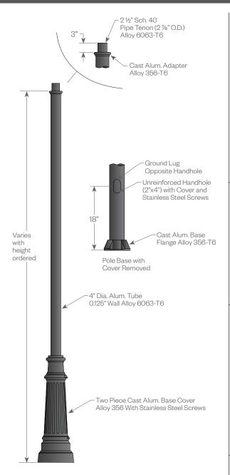
The post will be finished with an electrostatically applied thermoset polyester powder coat. Prior to finishing, the parts are thoroughly cleaned. Our powder coat finish is durable, long lasting, attractive and scratch resistant as well as environmentally friendly. We offer 7 stock finishes or hundreds of special order colors including custom matching for existing projects (additional charges apply).
