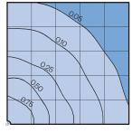
Typical HID light source 14,000 Lumens 12' Mounting Height Grid Spacing is 12'
