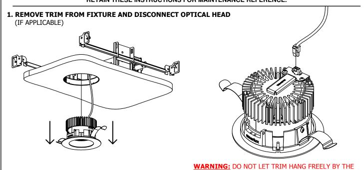
2. LOOSEN (2) SCREWS TO REMOVE OPTICAL HEAD AND REPLACE LENS
