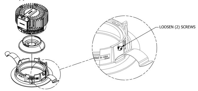
3. REINSTALL LENS, HEATSINK (POSITION AS SHOWN ABOVE), AND TIGHTEN SCREWS.
