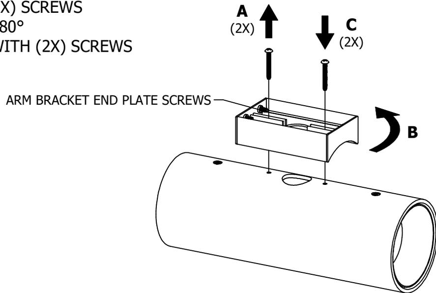
*\*THIS STEP IS OPTIONAL. ITS INTENT IS TO HIDE THE ARM BRACKET END PLATE SCREWS.*
