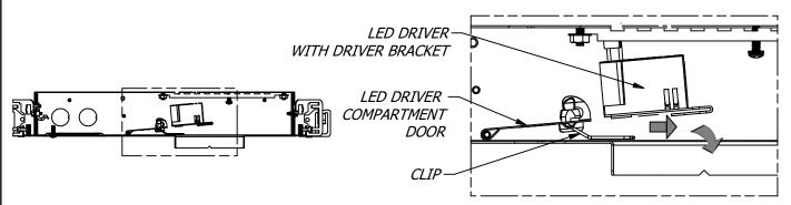
INSTALL NEW LED DRIVER ONTO THE DRIVER BRACKET. RECONNECT DRIVER WIRES, THEN SLIDE NEW DRIVER ONTO THE LED DRIVER COMPARTMENT DOOR. PUSH ALL WIRES DEEP INTO THE DRIVER COMPARTMENT AND THEN PUSH LED DRIVER DOOR UNTIL IT CLICKS INTO VERTICALLY POSITION.
