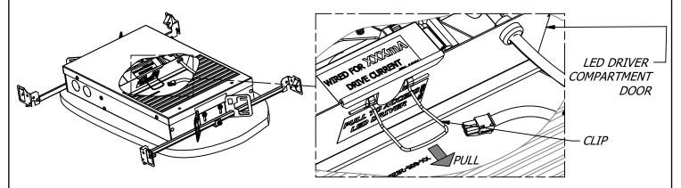
WHEN LED DRIVER COMPARTMENT DOOR IS IN HORIZONTAL POSITION, SLIDE THE LED DRIVER BRACKET OUT OF THE DOOR AND THEN PULL OUT OF THE HOUSING. DISCONNECT PRIMARY AND SECONDARY DRIVER WIRES.
