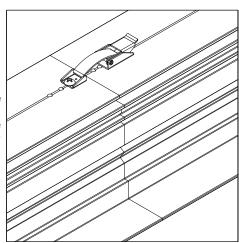
\*: Fixture MUST be mounted before ceiling is installed.
