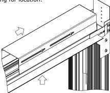
B. Loosen the 4 side screws to the Top Bracket. Slide Top Bracket to wall and tighten the 4 side screws. C. (Optional) Secure vertical and
