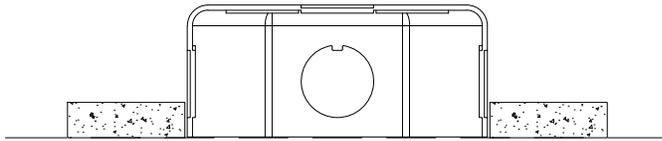
**Install junction boxes** - The junction boxes should be installed flush with ceiling plane as shown. This will ensure the canopy cover sits flush with the ceiling when install is finished.
