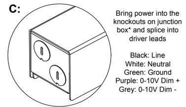
\*Driver Box size, shape & connection location may vary depending on fixture length and wattage. Most common box shown.
