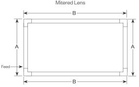
PR - Closed Rectangle, (4) straight lengths + (4) 90° corners Provide overall lengths: A' & B' Nomenclature: A-B-PR
