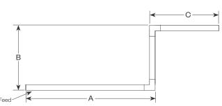
PZ - Open Z, (3) straight lengths + (2) 90° corners Provide overall lengths: A', B' & C' Nomenclature: A-B-C-PZ
