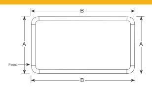
**PR** - Closed Rectangle, (4) straight lengths + (4) 90° corners *Provide overall lengths: A' & B'; Diameter*
