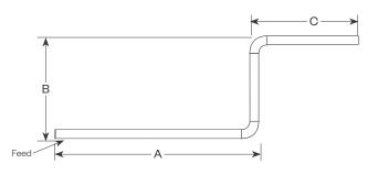
PZ - Open Z, (3) straights + (2) corners Provide overall lengths: A', B' & C', Diameter & Angle of corners Example: 12'x6'x10'.D36XA90.PZ
