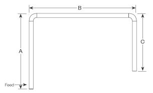
PU - Open U, (3) straights + (2) corners Provide overall lengths: A', B' & C'; Diameter & Angle of corners Example: 4'x10'.D72xA90.PU
