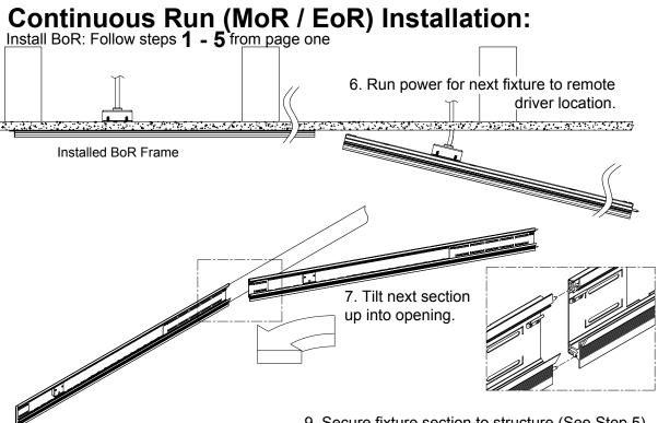
8. Slide section toward already installed fixture ensuring alignment pins insert into appropriate hole.
