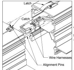
Joining the Housings Connect power from one fixture to the next using quick connects provided. Line up the two housings by using the alignment pins. Secure them together by using the Catch and Latch System on the top of the extrusion.
