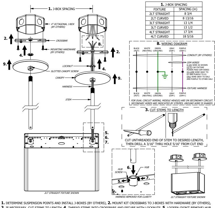
**3.** IF NECESSARY, CUT STEMS TO LENGTH, **4.** THREAD STEMS INTO CROSSBARS AND SECURE WITH LOCKNUTS, **5.** LOOSEN (DON'T REMOVE) HUB SCREWS (x4), **6.** FEED HARNESS THROUGH STEM AND INSERT STEMS INTO HUBS, **7.** TIGHTEN HUB SCREWS, **8.** WIRE ACCORDING TO LOCAL AND NATIONAL CODE, THEN **9.** SLIDE CANOPIES UP STEMS AND LOCK IN POSITION BY TIGHTENING SLOTTED CANOPY SCREWS.
