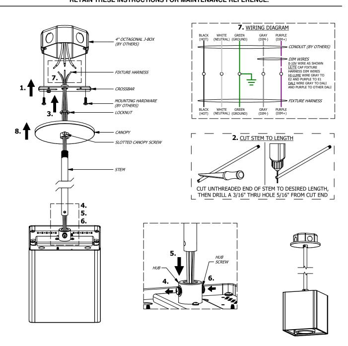
1. MOUNT KIT CROSSBAR TO J-BOX WITH HARDWARE (BY OTHERS), 2. IF NECESSARY, CUT STEM TO LENGTH, 3. THREAD STEM INTO CROSSBAR AND SECURE WITH LOCKNUT, 4. LOOSEN (DON'T REMOVE) HUB SCREWS (x2), 5. FEED HARNESS THROUGH STEM AND INSERT STEM INTO HUB, 6. TIGHTEN HUB SCREWS, 7. WIRE ACCORDING TO LOCAL AND NATIONAL CODE, THEN 8. SLIDE CANOPY UP STEM AND LOCK IN POSITION BY TIGHTENING SLOTTED CANOPY SCREW.
