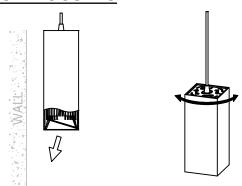
IF FIXTURE HAS WALL WASH TRIM AND/OR SQUARE HOUSING, ALIGN HOUSING BY HOLDING CORD THEN ROTATING HOUSING
