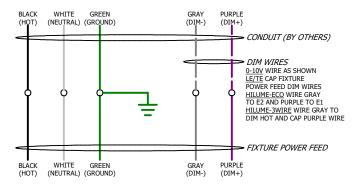
WIRE ACCORDING TO LOCAL AND NATIONAL CODE. CUT AND STRIP AS NEEDED. CAP UNUSED WIRES.
