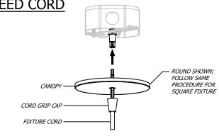
FEED FIXTURE CORD THROUGH CORD GRIP CAP, THEN CANOPY, THEN THROUGH CORD GRIP BASE, ADJUSTING FIXTURE OVERALL LENGTH (OAL)
