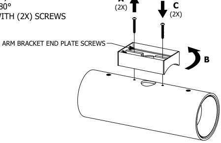
\*THIS STEP IS OPTIONAL. ITS INTENT IS TO HIDE THE ARM BRACKET END PLATE SCREWS.
