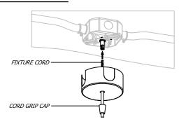
FEED FIXTURE CORD THROUGH CORD GRIP CAP, THEN CANOPY, THEN THROUGH CORD GRIP BASE, ADJUSTING FIXTURE OVERALL LENGTH (OAL)
