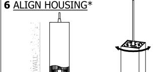
IF FIXTURE HAS WALL WASH TRIM AND/OR SQUARE HOUSING, ALIGN HOUSING BY HOLDING CORD THEN ROTATING HOUSING
