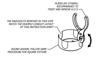
REMOVE CANOPY KNOCKOUTS TO MATCH CONDUIT LAYOUT
