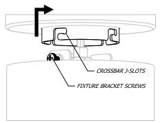
LOCATE FIXTURE BRACKET SCREWS IN CROSSBAR J-SLOTS, ROTATE UNTIL SCREWS ARE SEATED, THEN TIGHTEN SCREWS
