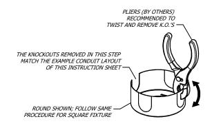
REMOVE CANOPY KNOCKOUTS TO MATCH CONDUIT LAYOUT
