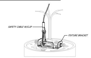
HOOK SAFETY CABLE CLIP ONTO FIXTURE BRACKET
