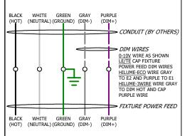
WIRE ACCORDING TO LOCAL AND NATIONAL CODE. CUT AND STRIP AS NEEDED. CAP UNUSED WIRES.
