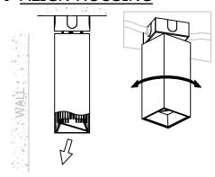
IF FIXTURE HAS WALL WASH TRIM AND/OR SQUARE HOUSING, SIMPLY ROTATE HOUSING (100° MAX.)
