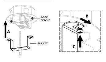
ATTACH BRACKET TO J-BOX SCREWS, THEN TIGHTEN SCREWS
