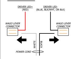
WIRE DRIVER LED +/- WIRES TO POWER CORD WIRES WITH WAGOS
