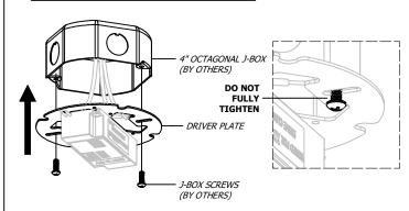
MOUNT DRIVER PLATE TO J-BOX WITH SCREWS (BY OTHERS). DO NOT FULLY TIGHTEN SCREWS
