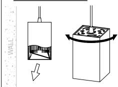
IF FIXTURE HAS WALL WASH TRIM AND/OR SQUARE HOUSING, ALIGN HOUSING BY HOLDING CORD THEN ROTATING HOUSING
