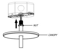
SLIP CANOPY ONTO STEM, THREAD NUT ONTO STEM, FEED HARNESS THROUGH CROSSBAR, THREAD STEM INTO CROSSBAR, THEN TIGHTEN NUT
