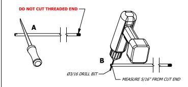
IF NECESSARY, CUT END WITH THRU HOLE TO DESIRED LENGTH, THEN DRILL A Ø3/16" THRU HOLE 5/16" FROM END
