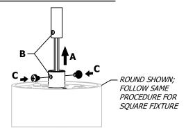
FEED FIXTURE HARNESS THROUGH STEM, ALIGN STEM HOLES TO (2x) HUB SCREWS, THEN TIGHTEN SCREWS
