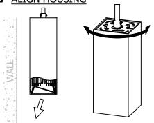
IF FIXTURE HAS WALL WASH TRIM AND/OR SQUARE HOUSING, ALIGN HOUSING BY HOLDING STEM THEN ROTATING HOUSING
