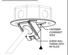
HINGE MP PLATE INSIDE CROSSBAR, SLIDE TO ALIGN HOLES, THEN FASTEN MP PLATE TO CROSSBAR WITH SCREW
