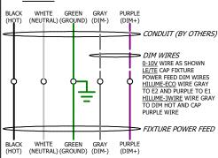
SUPPORT FIXTURE THROUGHOUT WIRING PROCESS. WIRE ACCORDING TO LOCAL AND NATIONAL CODE. CUT AND STRIP AS NEEDED, CAP UNUSED WIRES.
