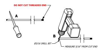
IF NECESSARY, CUT END WITH THRU HOLE TO DESIRED LENGTH, THEN DRILL A  $\emptyset 3/16$ " THRU HOLE 5/16" FROM END
