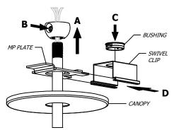
FEED HARNESS/STEM THROUGH CANOPY AND MP PLATE, THREAD STEM INTO HALF BALL, THEN TIGHTEN SCREW. INSERT BUSHING INTO SWIVEL CLIP THEN SLIDE ONTO MP PLATE.
