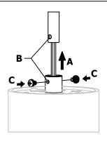
FEED FIXTURE HARNESS THROUGH STEM, ALIGN STEM HOLES TO (2x) HUB SCREWS, THEN TIGHTEN SCREWS
