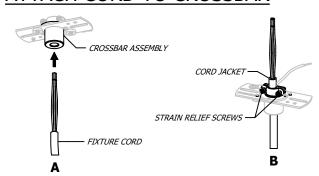
FEED FIXTURE CORD THROUGH KIT CROSSBAR ASSEMBLY, THEN TIGHTEN SRAIN RELIEF SCREWS ON CORD JACKET, ADJUSTING FIXTURE OVERALL LENGTH (OAL)
