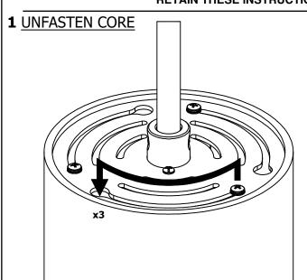
LOOSEN BUT DON'T REMOVE (3x) CORE SCREWS ON TOP OF CYLINDER, ROTATE CORE 90° CLOCKWISE, THEN DROP CORE THROUGH KEYSLOTS WHILE SUPPORTING CORE
