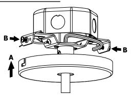
A RAISE CANOPY AND TWIST INTO PLACE, THEN B TIGHTEN (2x) CANOPY SCREWS
