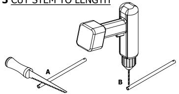
IF NECESSARY, A CUT ONE END TO DESIRED LENGTH, THEN B DRILL A Ø3/16" THRU HOLE 5/16" FROM END
